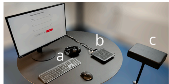
Fig. 3. The setup in the first study, consisting of (a) a screen, keyboard, mouse and headphones; (b) the mid-air haptics device STRATOS Explore and Leap Motion controller; (c) and an armrest.
